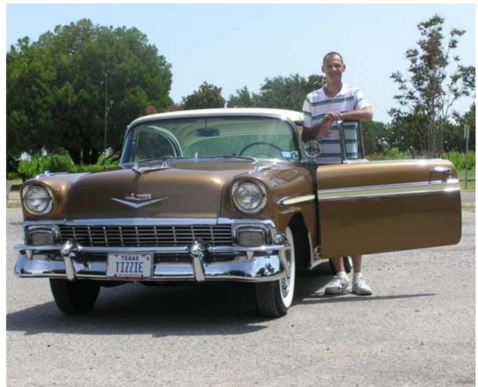
could do and Mom supervised. All rubber bushings for the control arms, steering linkage and rear springs were replaced along with the shocks. She needed new tires and I stayed with the bias ply because I think they have the correct look.
