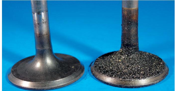
**The valve on the left is clean, while the valve on the right has fuel-related deposits that will lower engine performance. Burning the best fuel possible in your Chevy can save your engine from detrimental damage like this.**
