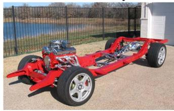
in St. Joseph, MO. The suspension is not damaged and it has everything - brakes, rack and pinion, suspension cradle, complete rear end, everything for \$1250. \$200 more and it's strapped to a pallet and it's here three days later. Homer and I start tearing it apart immediately. The front suspension cradle goes to Newman's where it will be mated with the new frame. I start polishing the Vette A-arms and all those other pieces that make up the suspension.
